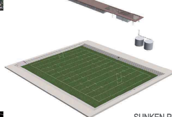
SUNKEN PLAYING FIELD WITH DRIP LINE IRRIGATION
