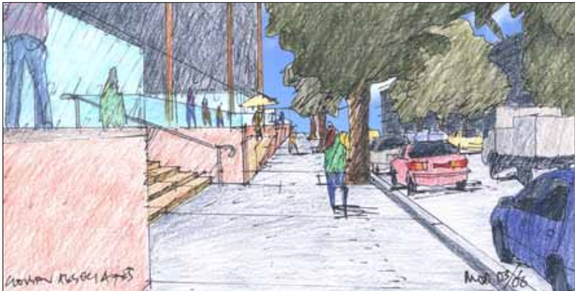
Artist's impression of Mitchell Road looking north with required steps / ramps to access the floor level 1.5m above existing pavements.
