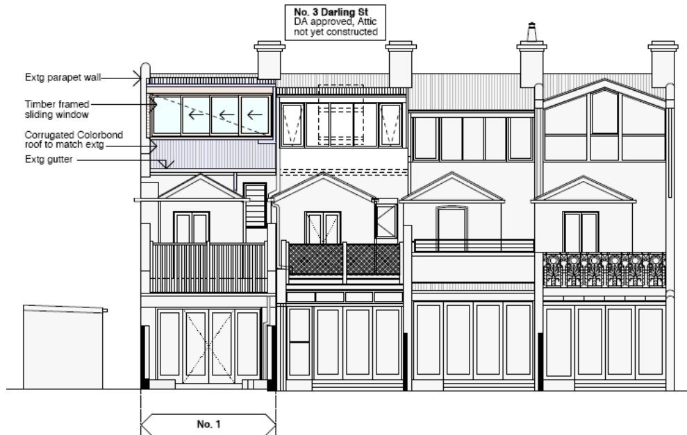
Figure 6 – Proposed rear (Northeast) elevation (as amended).
