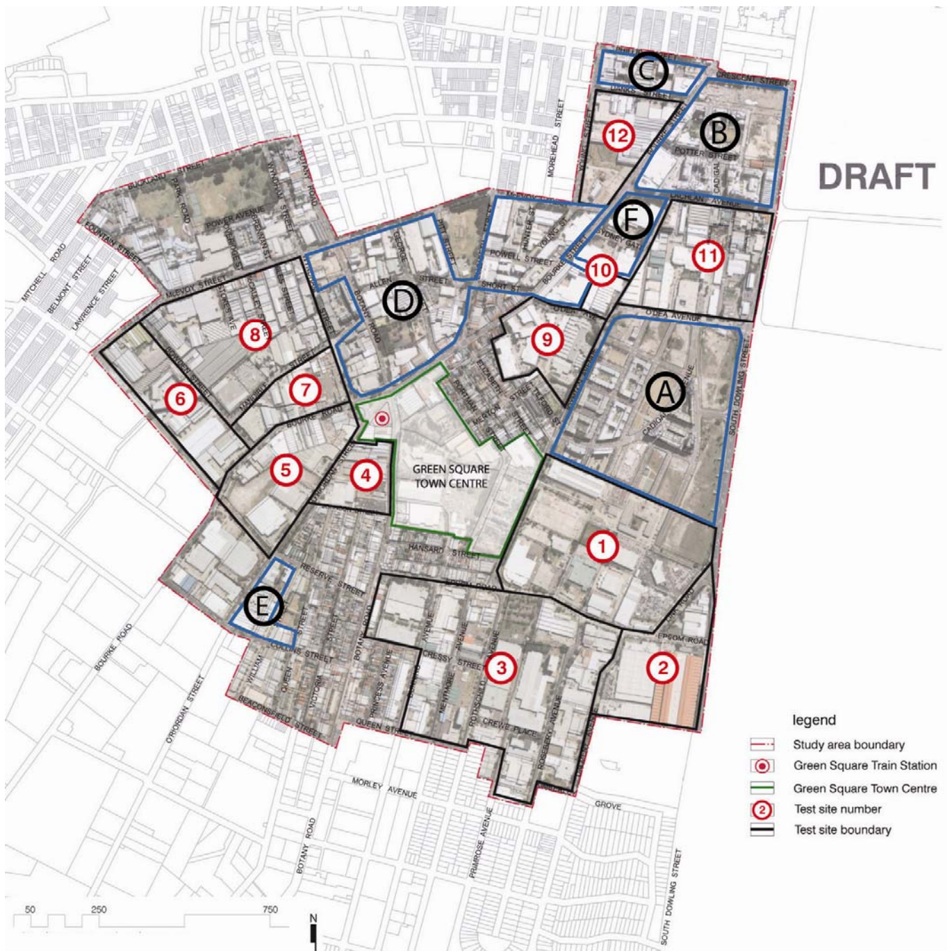
Figure 255 Development potential areas This plan references the site tests (1-12) and the areas (A-E) which are included in the development potential assessment of the study area.
