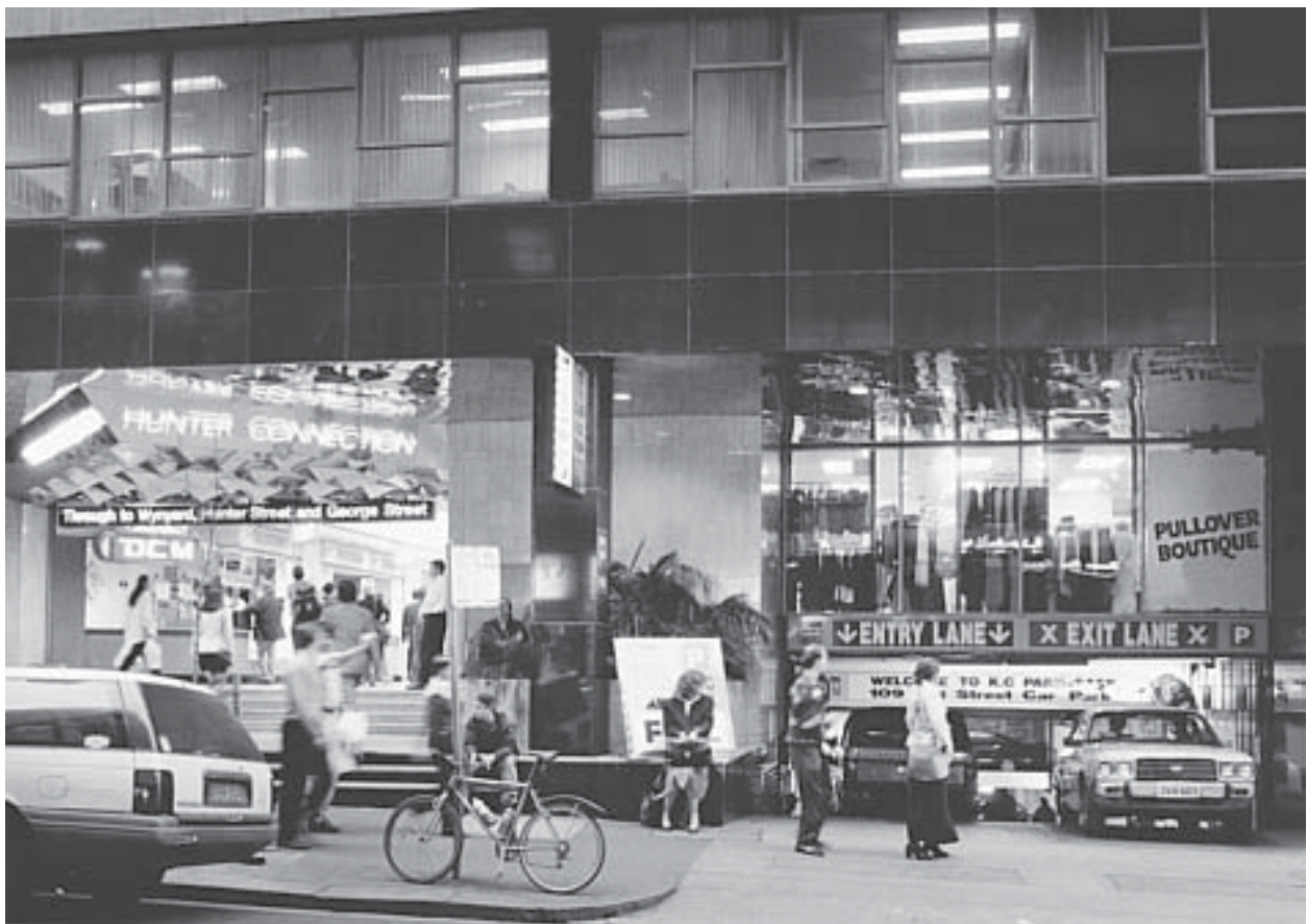
Active uses or items of visual interest are appropriate above vehicle access points (ie, in the horizontal line of sight of a pedestrian).
