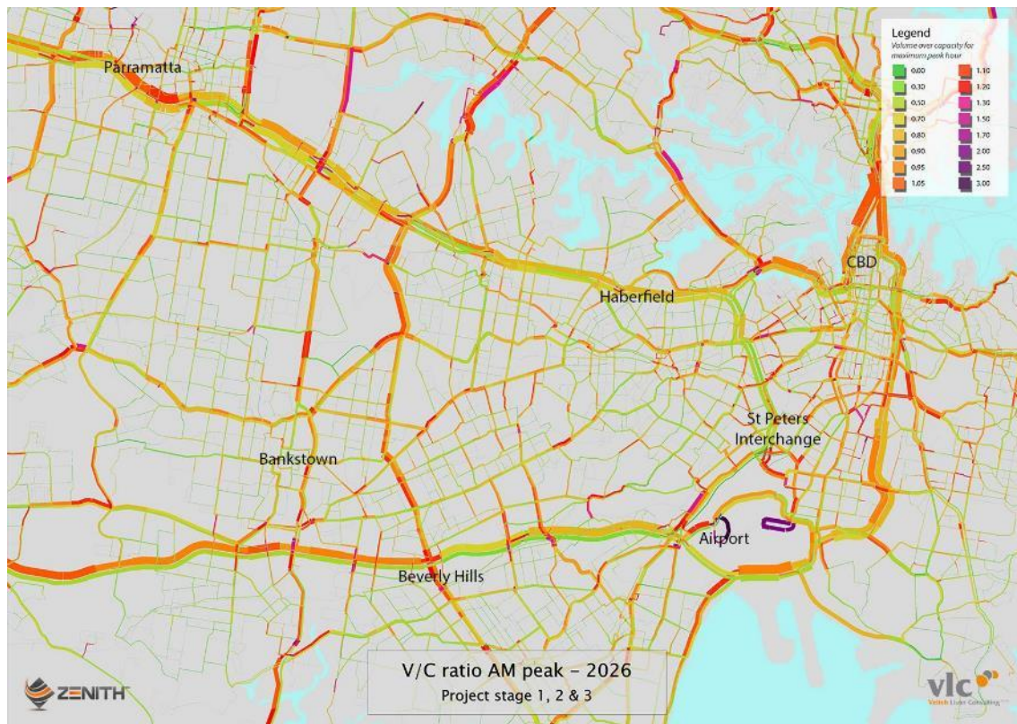
FIGURE 4 VOLUME TO CAPACITY RATIO 2026 WITH WESTCONNEX STAGES 1, 2 & 3
