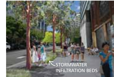
Photomontage showing possible stormwater infiltration beds (rain gardens) along Quay Street
