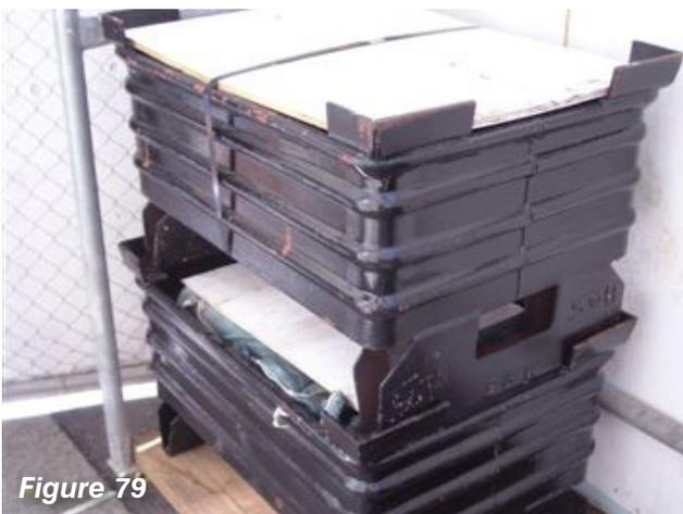
**Figure 78:** Typical concrete block counterweight with lateral bracings.
