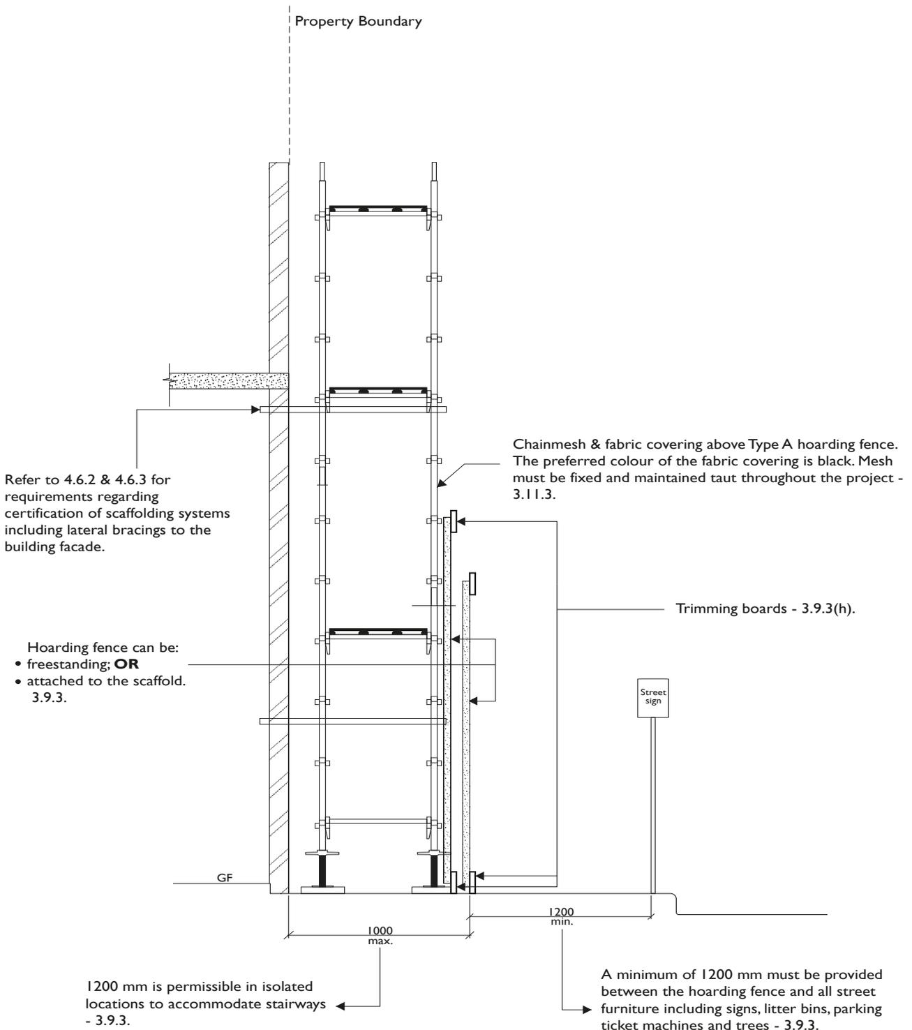
**Figure 128:** Elevation showing the key design features for scaffolding and 'Type A' hoardings.
