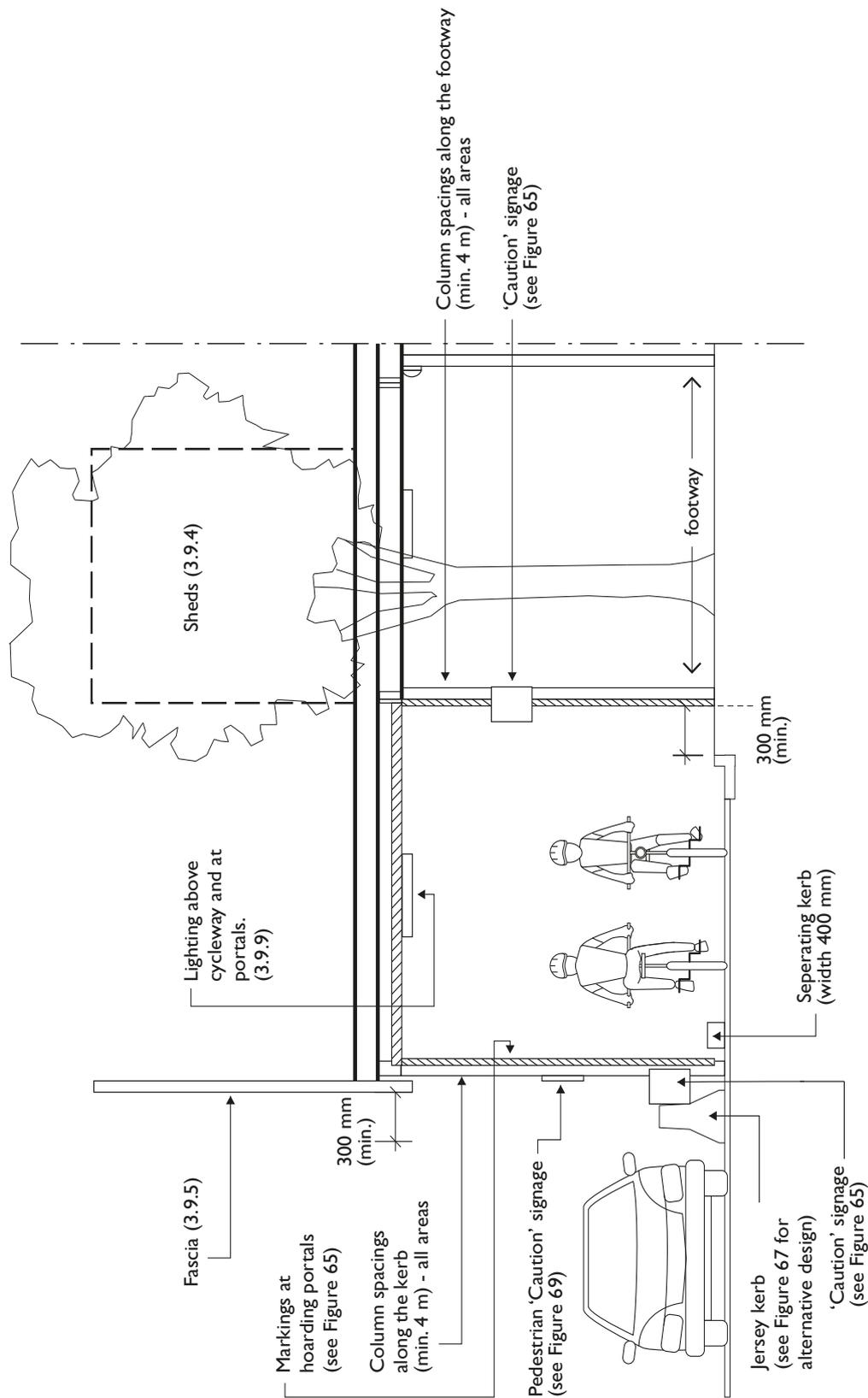
**Figure 67:** Alternative Type B hoarding design for installation over a cycleway where, due to local road and traffic conditions, it is not possible to comply with the standard design in Figure 66.
