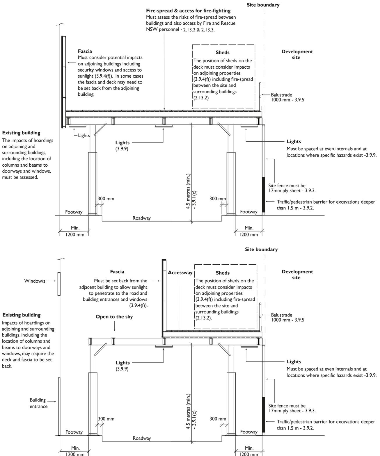
**Figure 58 (a) (top):** Section detail of a 'Type B' hoarding erected over a roadway. Potential impacts on adjoining properties and on vehicles including vehicle access to driveways must be considered in the design.
