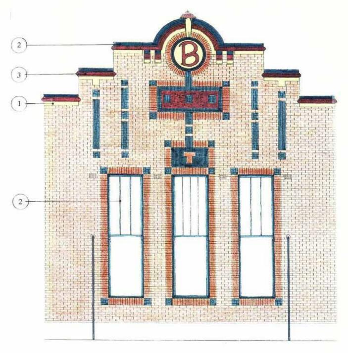
Do not paint face brickwork or tile wall surfaces
