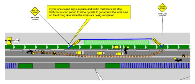
Traffic controllers can stop traffic flow in both directions to enable people riding to divert onto the roadway without risking collision with moving traffic. Ensure this works in both directions and is well signed. Only works with traffic controllers present and is not to be left overnight.
