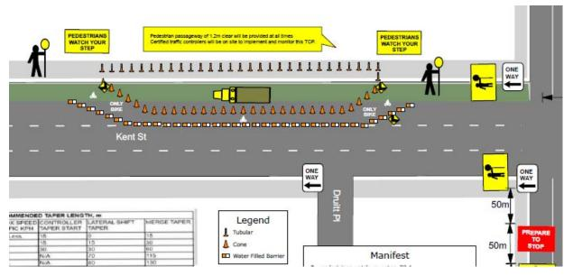
Divert both directions of bike traffic onto a protected area of the road with water filled barrier separation using a parking or traffic lane. You may need to remove the far side parking lane or divert motor traffic to create space. Use a safe driveway or kerb ramp (no lips) for entry/exit. Ensure it works in both directions, is well signed and the surface is smooth and clean. Minimum width is 2.5-3m for a two way path or 1.5-2m for one way lane or path.
