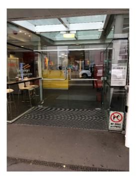
The pathway to the main pedestrian entrance includes a shallow descent from the footpath to the KGV entrance. KGV has step free access. The doorway includes heavy double swing glass doors at entry. Doors have fixed bar to pull open. Single door opens to 1020mm wide.
