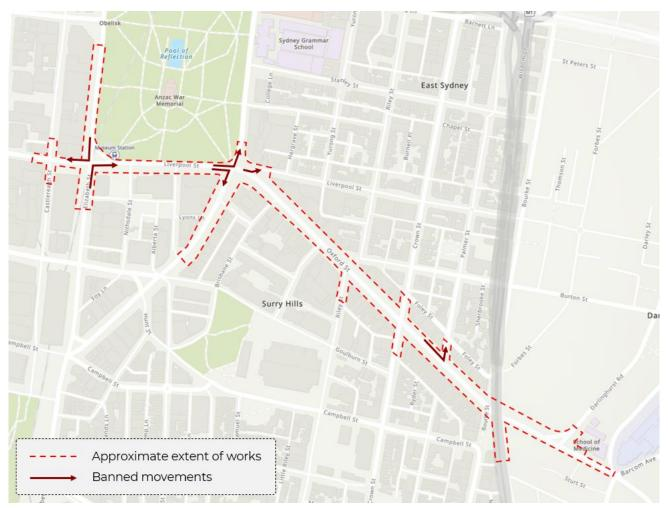
Figure 5.13 Summary of banned movements resulting from required operational changes
