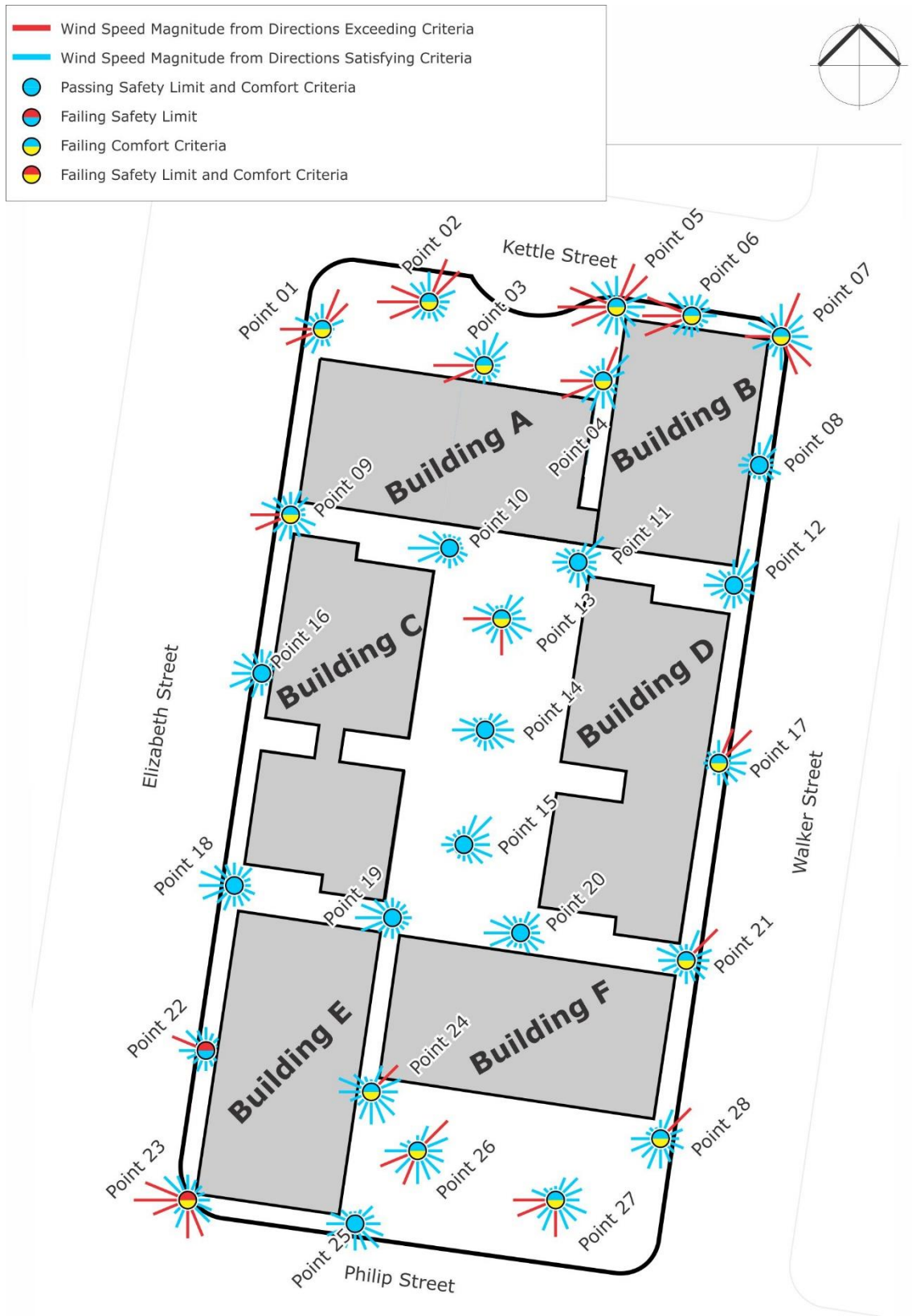
Figure 7a: Wind Tunnel Results – Ground Floor (results shown without treatments applied)
