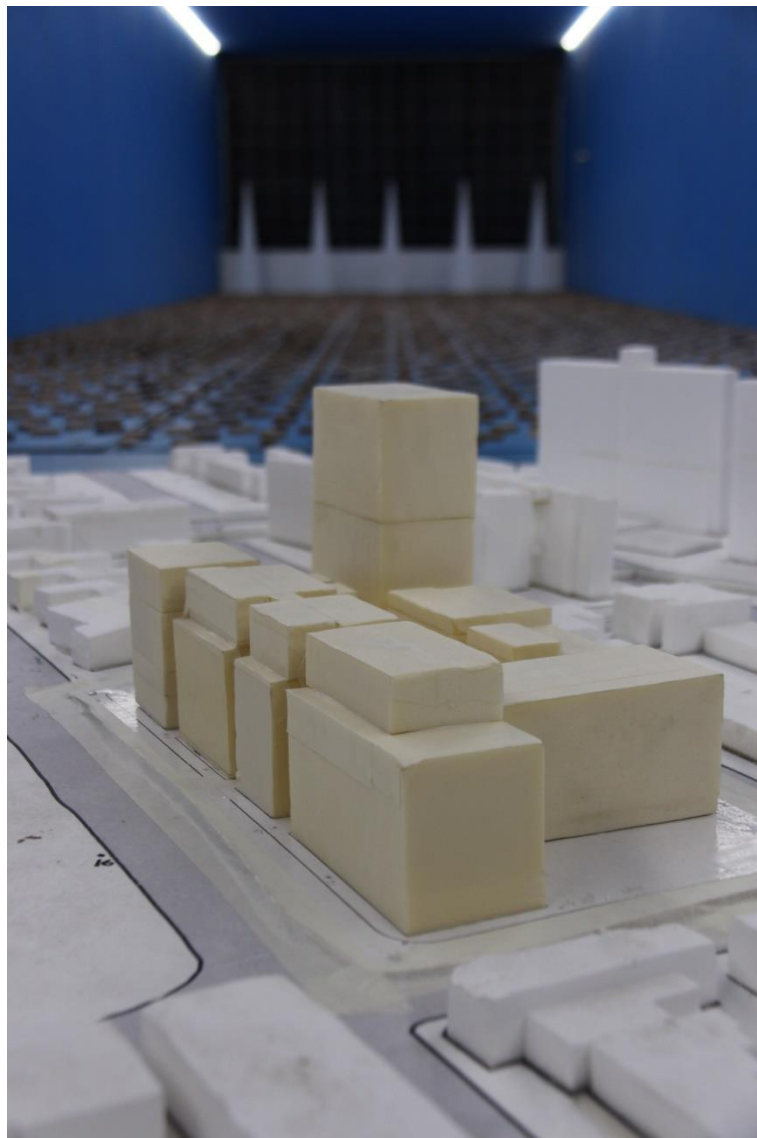
Figure 2a: Photograph of the Wind Tunnel Model (proposed scenario, view from the north-east)
