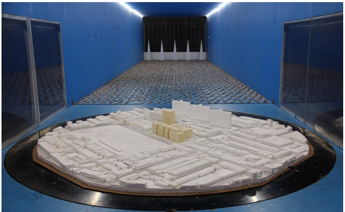
Figure 2c: Photograph of the Wind Tunnel Model (proposed scenario, view from the south-west)
