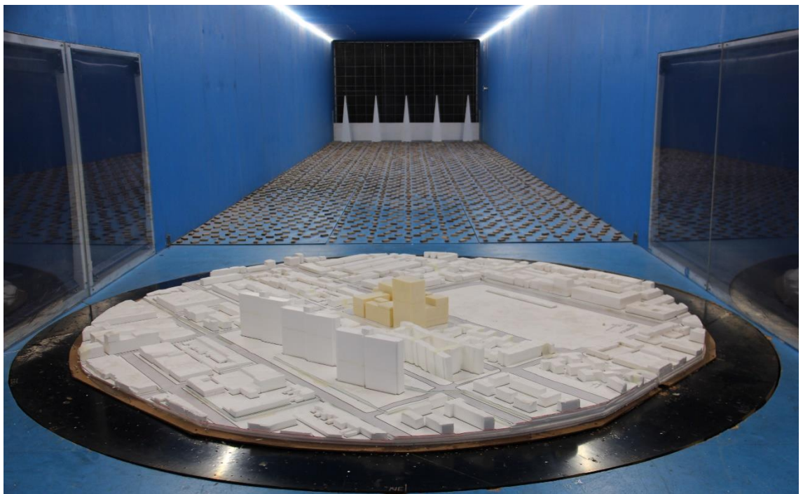
Figure 2e: Close up photograph of the Wind Tunnel Model (proposed scenario, view from the north-east)
