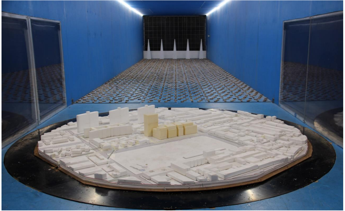
Figure 2d: Close up photograph of the Wind Tunnel Model (proposed scenario, view from the north-west)
