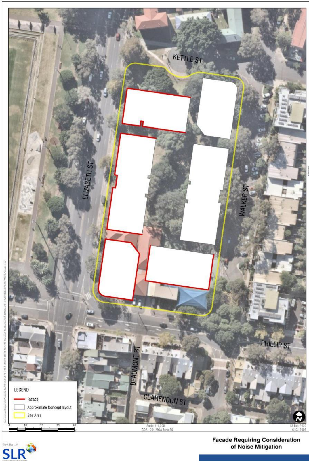
Figure 8 Facades Requiring Consideration of Noise Mitigation
