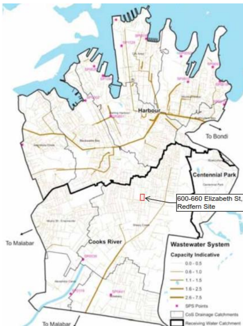
Figure 9: Wastewater Network System (CoS Decentralised Water Masterplan, 2012)
