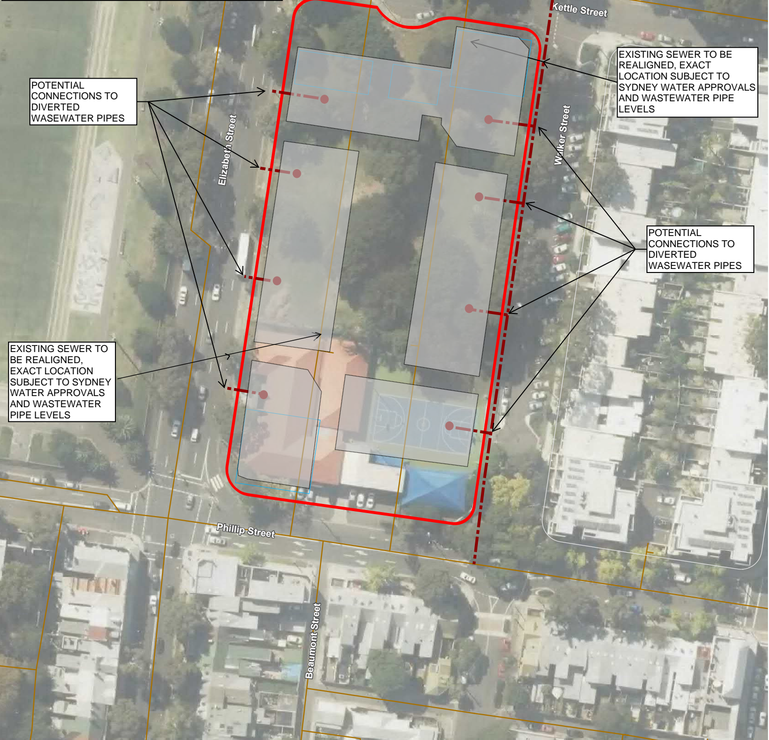
FIGURE 11 - WASTEWATER PLAN (ASSUMING SEPERATE BUILDING CONNECTIONS)
