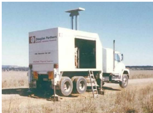
Figure 2: Purpose built CPT rig
