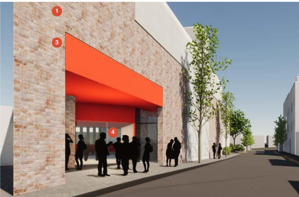
Figure 184: Perspective - Main entrance on Nimrod Street. Recycled brickwork facade (1), new integrated signage above entry (3) and new under cover entrance for the congregating public connected to the new public space (4).
