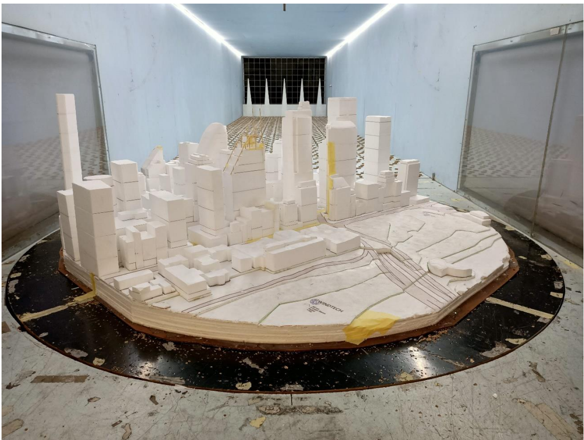
Figure 1a: Photograph of the Wind Tunnel Model (Existing Scenario, view from the south-east)
