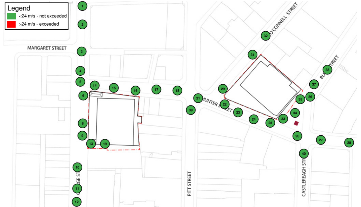
189. Irwin Sensor Safety Results for Proposed Development (Source: Sydney Metro Wes Pedestrian Wind Assessment)
