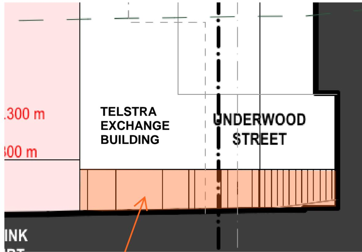
Public easement to extend to height of existing Telstra Colonnade soffit. Height varies.
