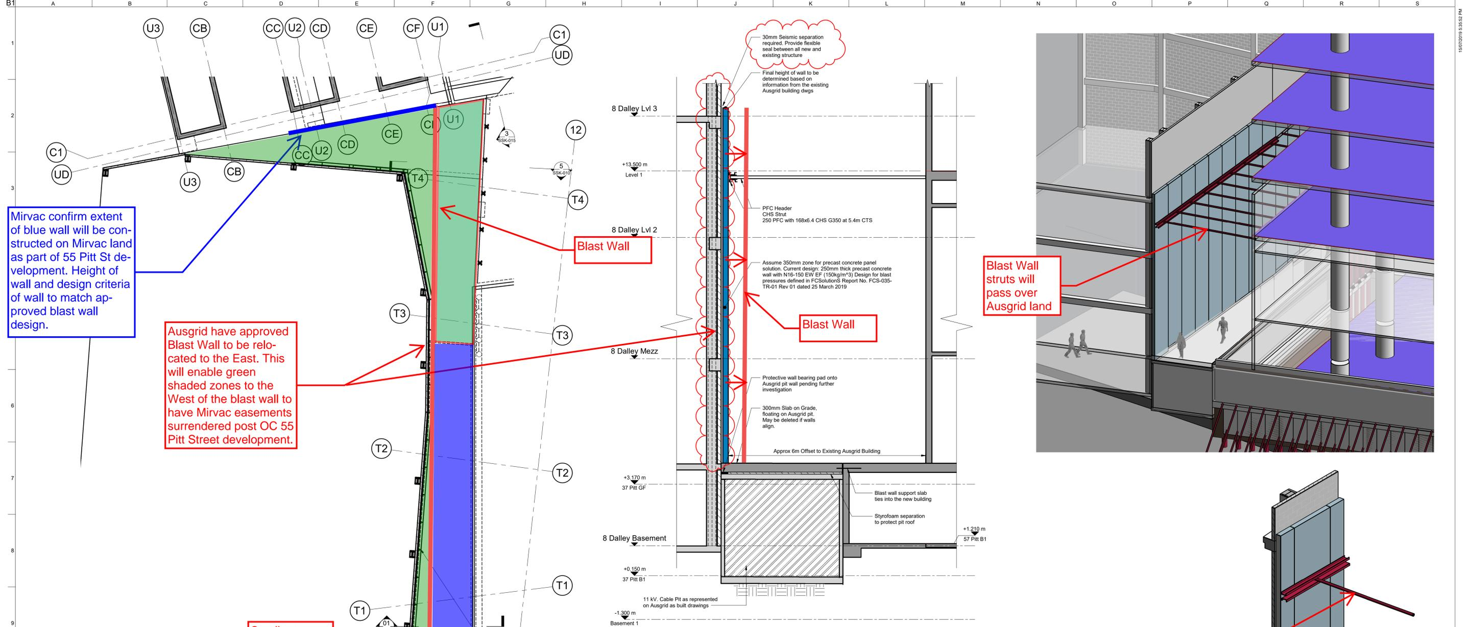
Mirvac confirm extent of blue wall will be constructed on Mirvac land as part of 55 Pitt St development. Height of wall and design criteria of wall to match approved blast wall design.
