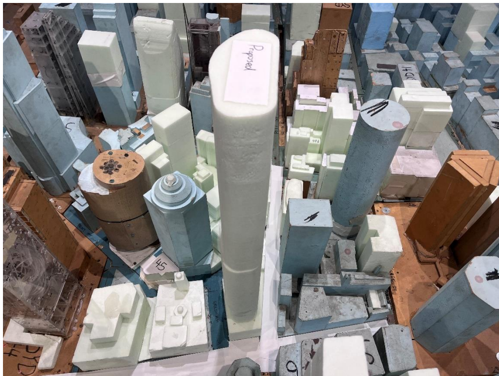
Figure 3b – View from the north of the 1/400 scale model of the 56 Pitt Street – Proposed Configuration (February 2024 Design) in the wind tunnel.
