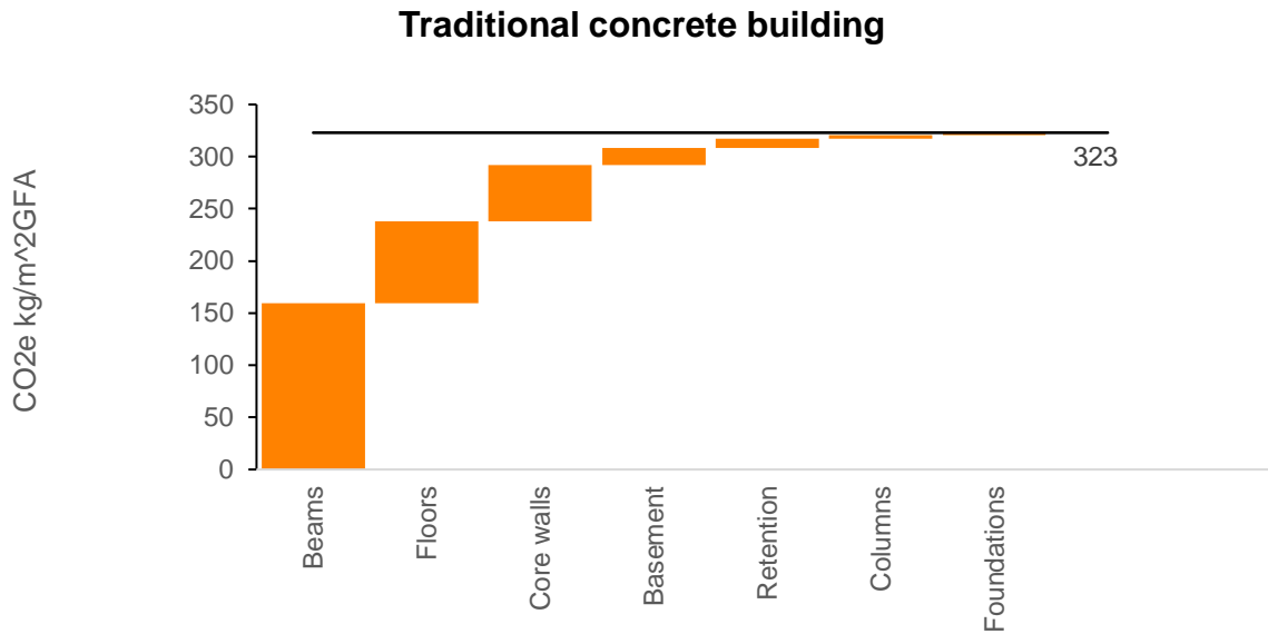
Figure 1: Embodied carbon for the structure of a traditional concrete building
