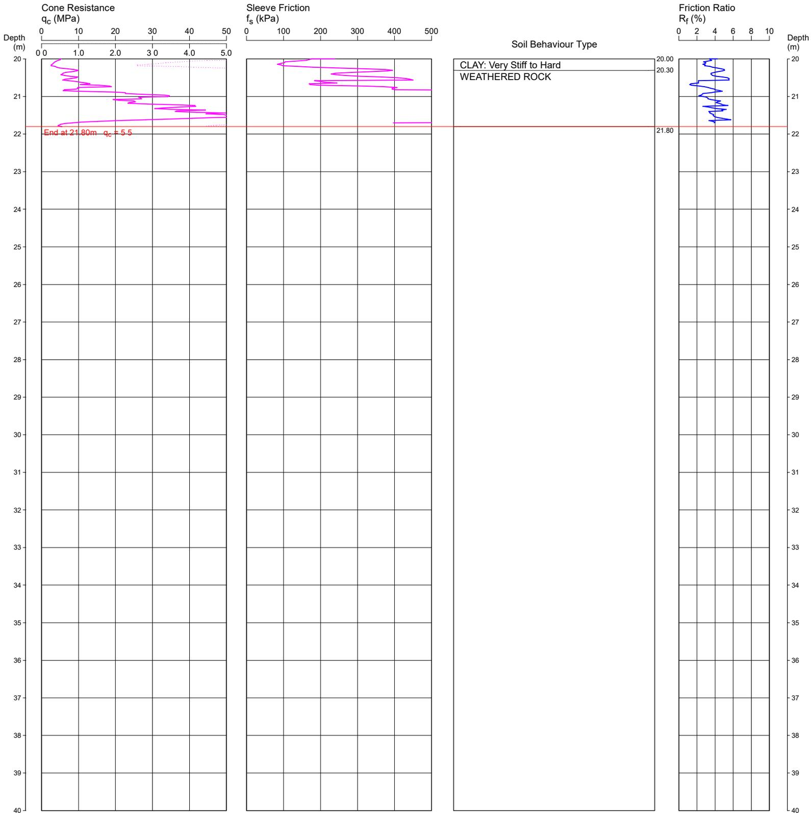
REMARKS CONCRETE DEPTH 150MM. GROUNDWATER MEASURED AT 4.2M DEPTH AFTER REMOVAL OF RODS.
