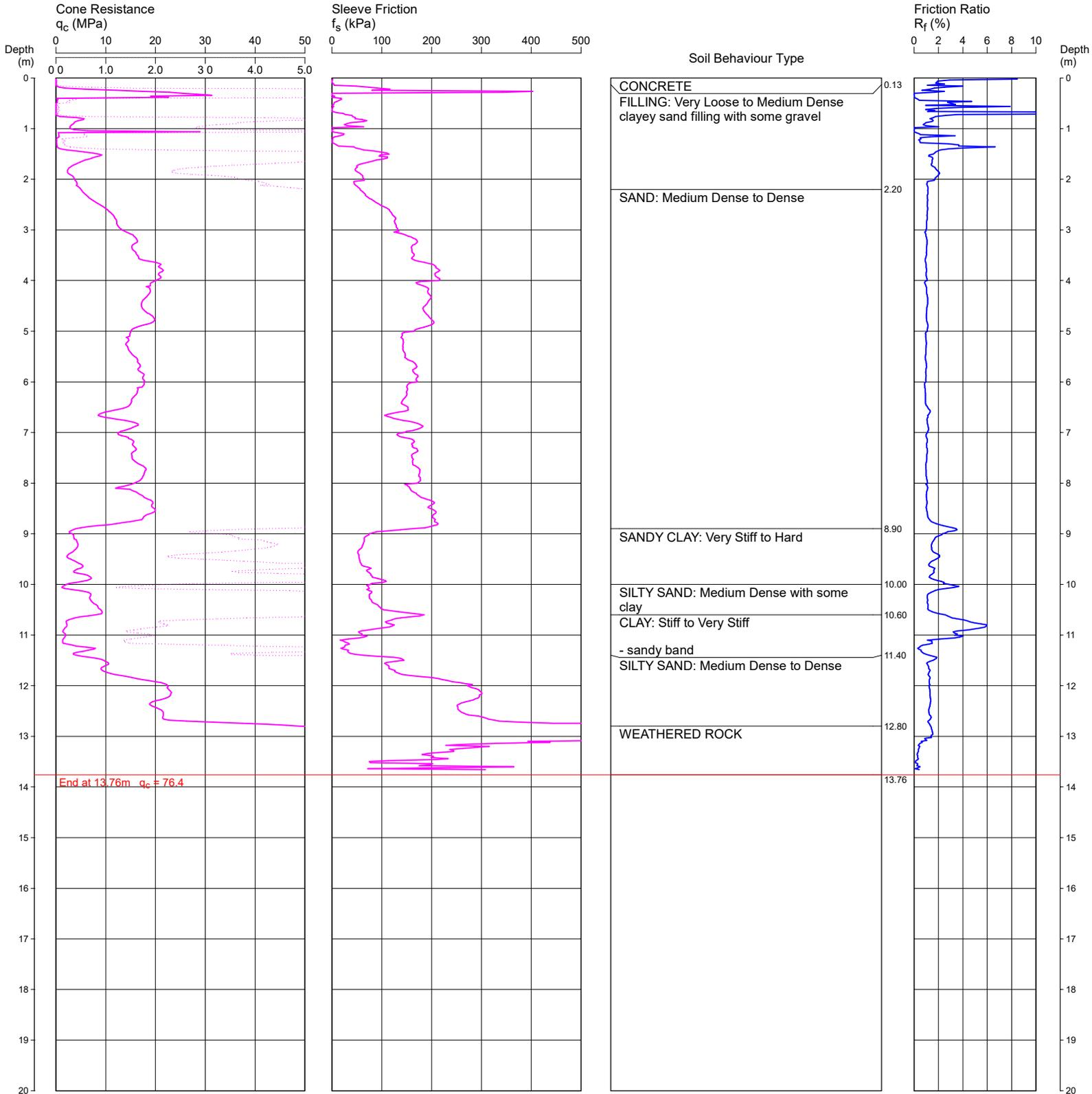
REMARKS DUMMY CONE FROM 0.38M TO 0.8M AND 1.06M TO 1.5M DEPTHS.
