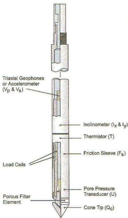
Figure 1: Cone Diagram
