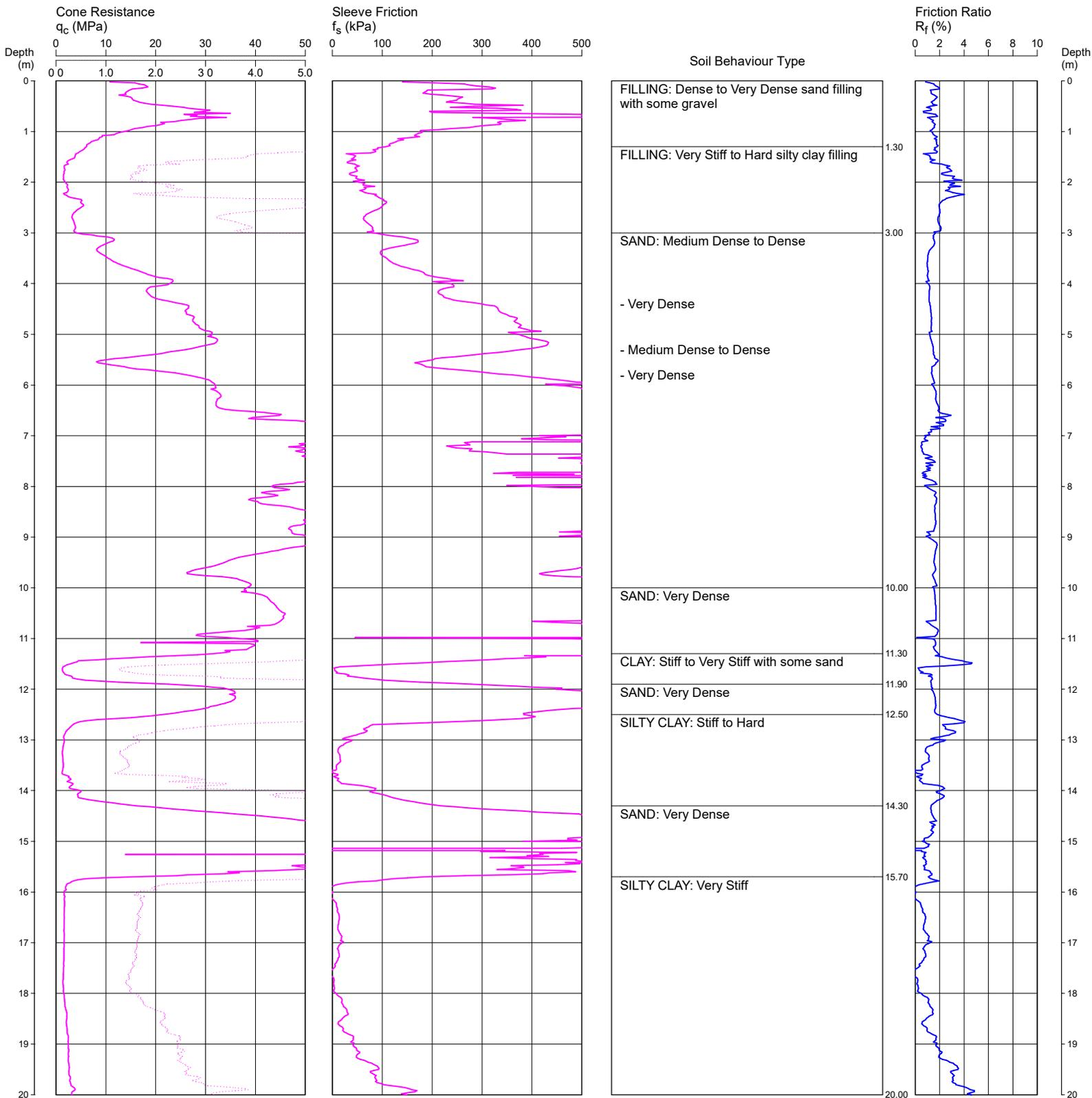
REMARKS GROUNDWATER MEASURED AT 4.9M DEPTH AFTER REMOVAL OF RODS.
