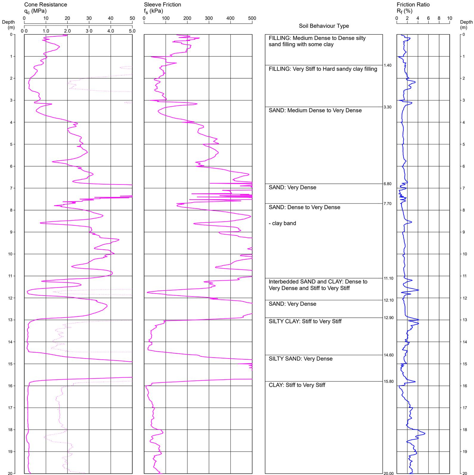
REMARKS HOLE COLLAPSE MEASURED AT 5.0M DEPTH AFTER REMOVAL OF RODS.
