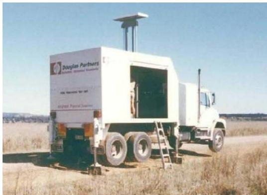
Figure 2: Purpose built CPT rig
