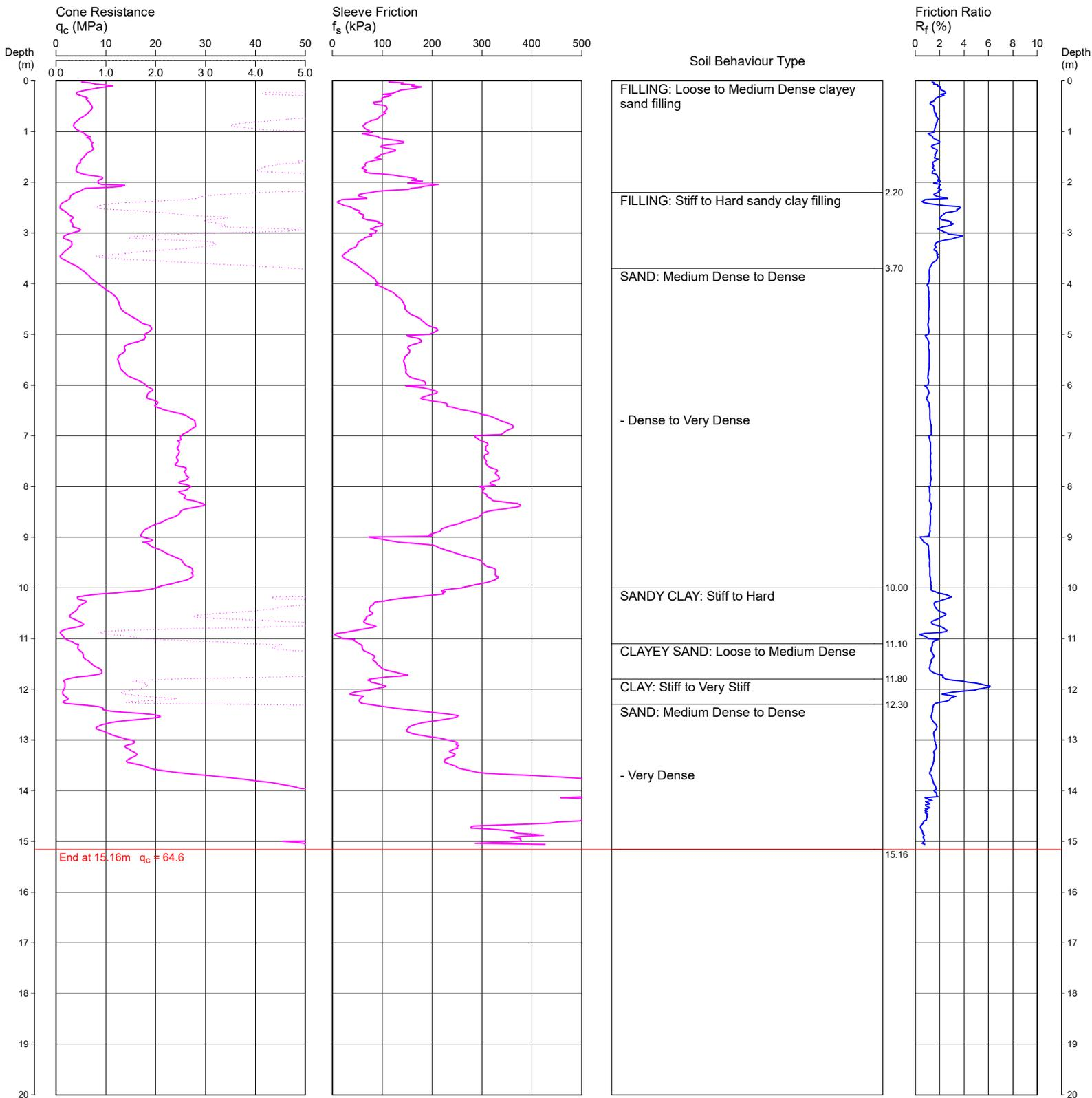
REMARKS TEST ENDED DUE TO TRUCK L FT NG. HOLE COLLAPSE MEASURED AT 5 M DEPTH AFTER REMOVAL OF RODS.
