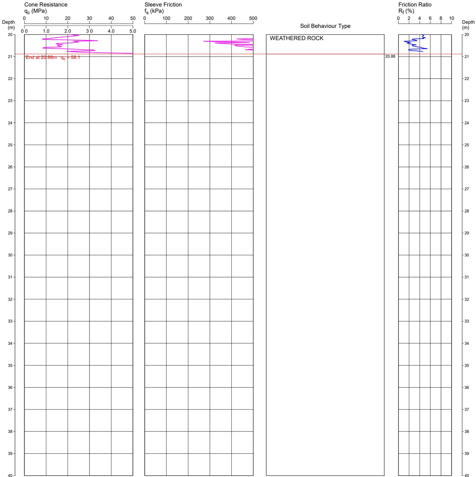
REMARKS DUMMY CONE FROM 1.0M TO 1 5M DEPTH. HOLE COLLAPSE MEASURED AT 6.0M DEPTH AFTER REMOVAL OF RODS.
