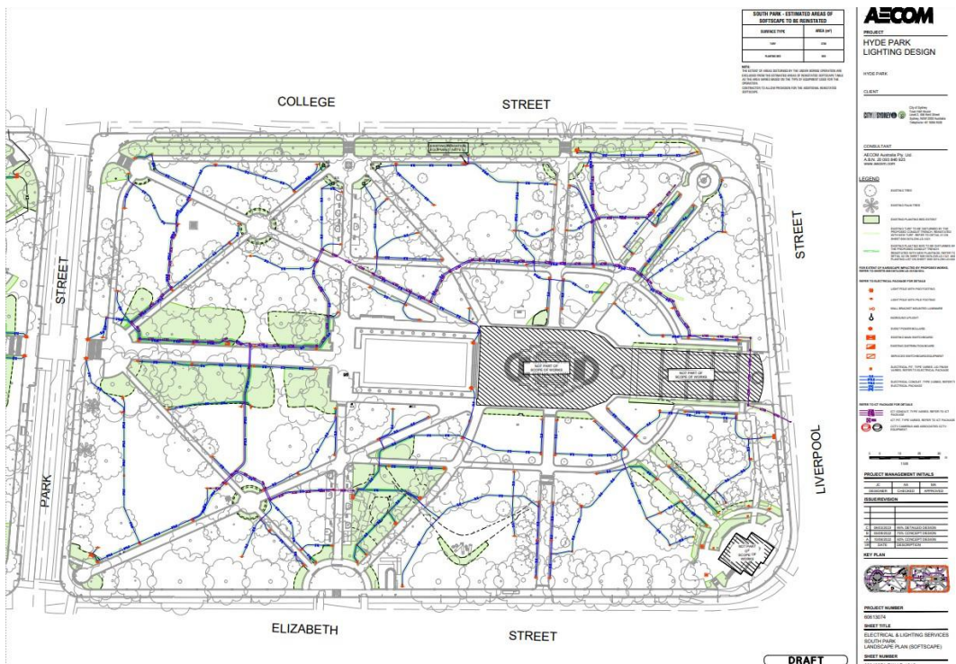
Figures 6.4 and 6.5 Hyde Park north and south landscape drawings 60613074-DW-LD-1011-12 showing landscape, power and reticulation layout, including locations of Lumieres and event power bollards. New underground cabling is indicated in blue. (Source: AECOM March 2023)
