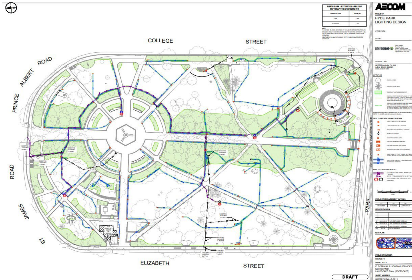
Figure 3.1 Hyde Park North landscape drawing 60613074-DW-LD-1011 showing landscape, power and reticulation layout, including locations of Lumieres and event power s. New underground cabling is indicated in blue. (Source: AECOM 2023)
