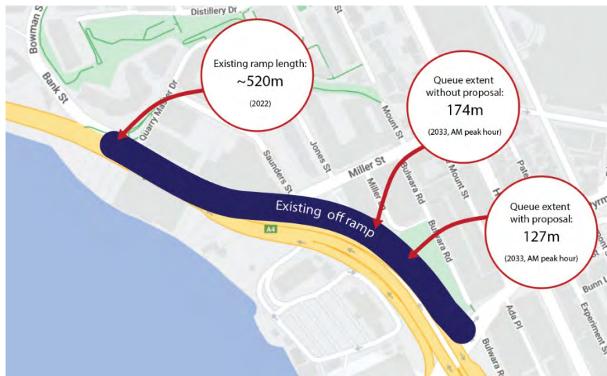
Figure 1 Exit ramp length for the AM peak with and without the proposal.
