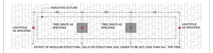
REFER TO DRAWING 2.2.1 FOR GRANITE PAVING LINKED TREE PIT PLAN
