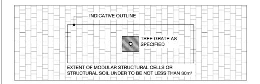
REFER TO DRAWING 2.2.1 FOR GRANITE PAVING SINGLE TREE PIT PLAN
