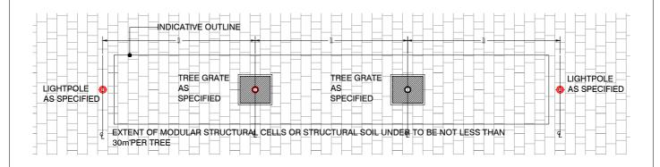
REFER TO DRAWING 2.2.1 FOR GRANITE PAVING LINKED TREE PIT PLAN
