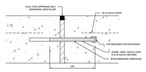
NOTE: BOND-BREAKING COMPONENT AND END CAP MAY BE REPLACED WITH A PURPOSE-MADE DOWEL SLEEVE.
