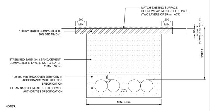
$^*$ 1. AREAS LESS THAN 10 m² - IF THE ROAD BASE IS USED INSTEAD OF CEMENT STABILISED SAND, THE TOP 100 mm OF DGB CAN BE SCARIFIED AND RECOMPACTED IF THE MATERIAL IS FOUND TO COMPLY WITH STANDARD
