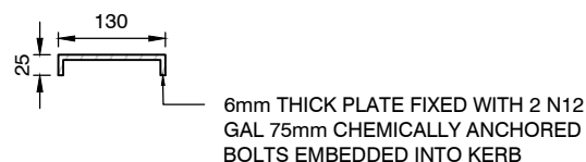
GALVANISED PLATE DETAIL 1:10
