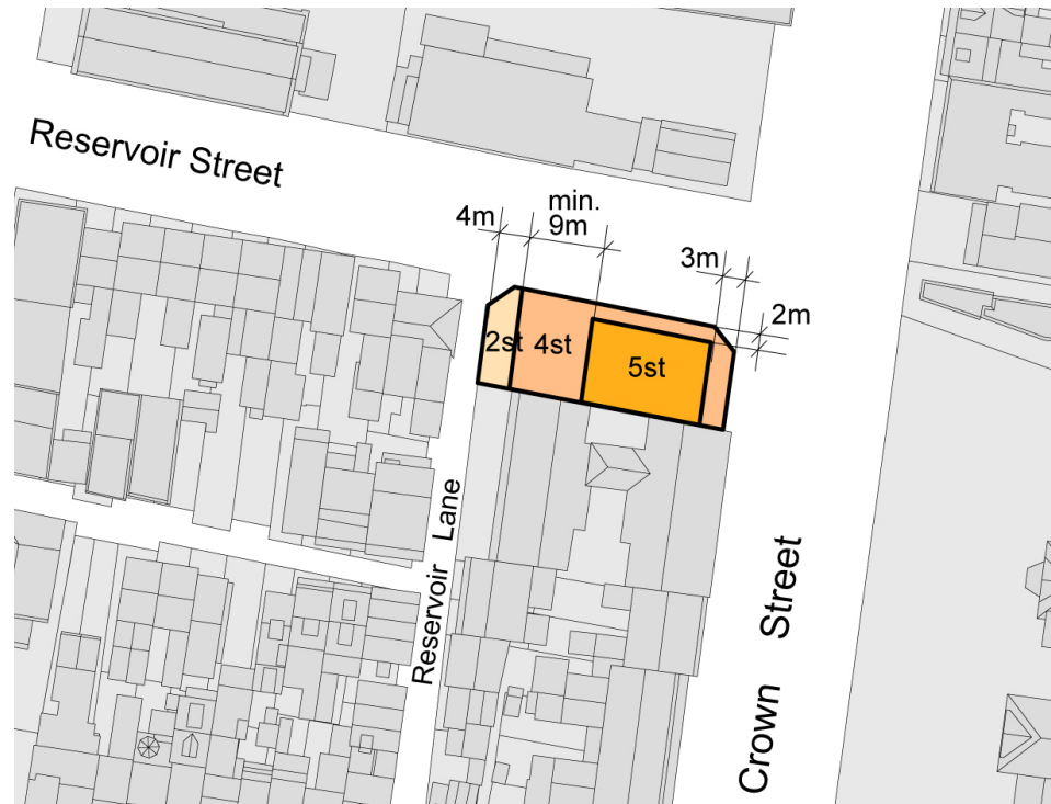
Figure 6.89 Height in storeys for 287-289 Crown Street, Surry Hills
