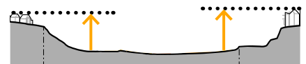
Figure 17: In principle, the height of buildings is equivalent to the height of surrounding development.
