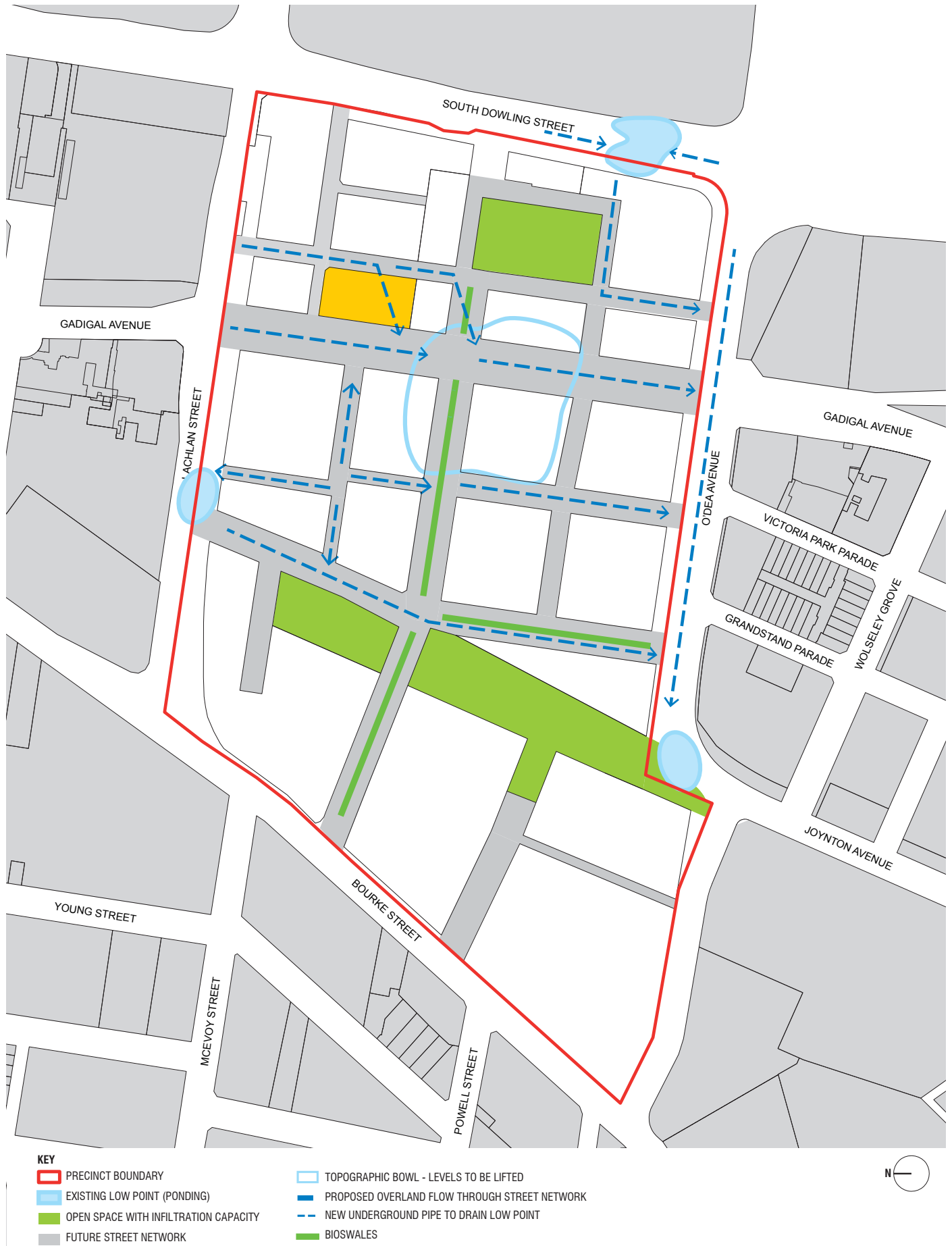
Figure 5.106 Lachlan Precinct Stormwater Management
