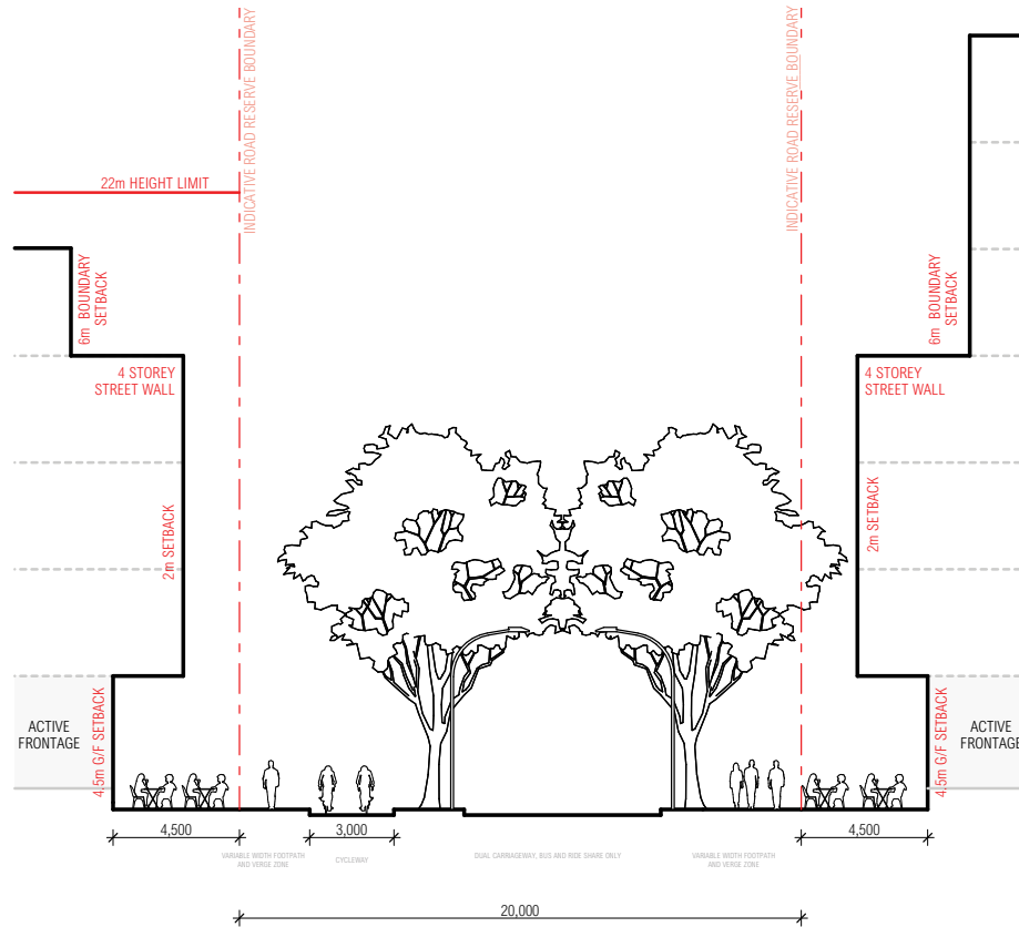
Figure 5.224 Indicative street section – Ashmore Connector West, North Alexandria
