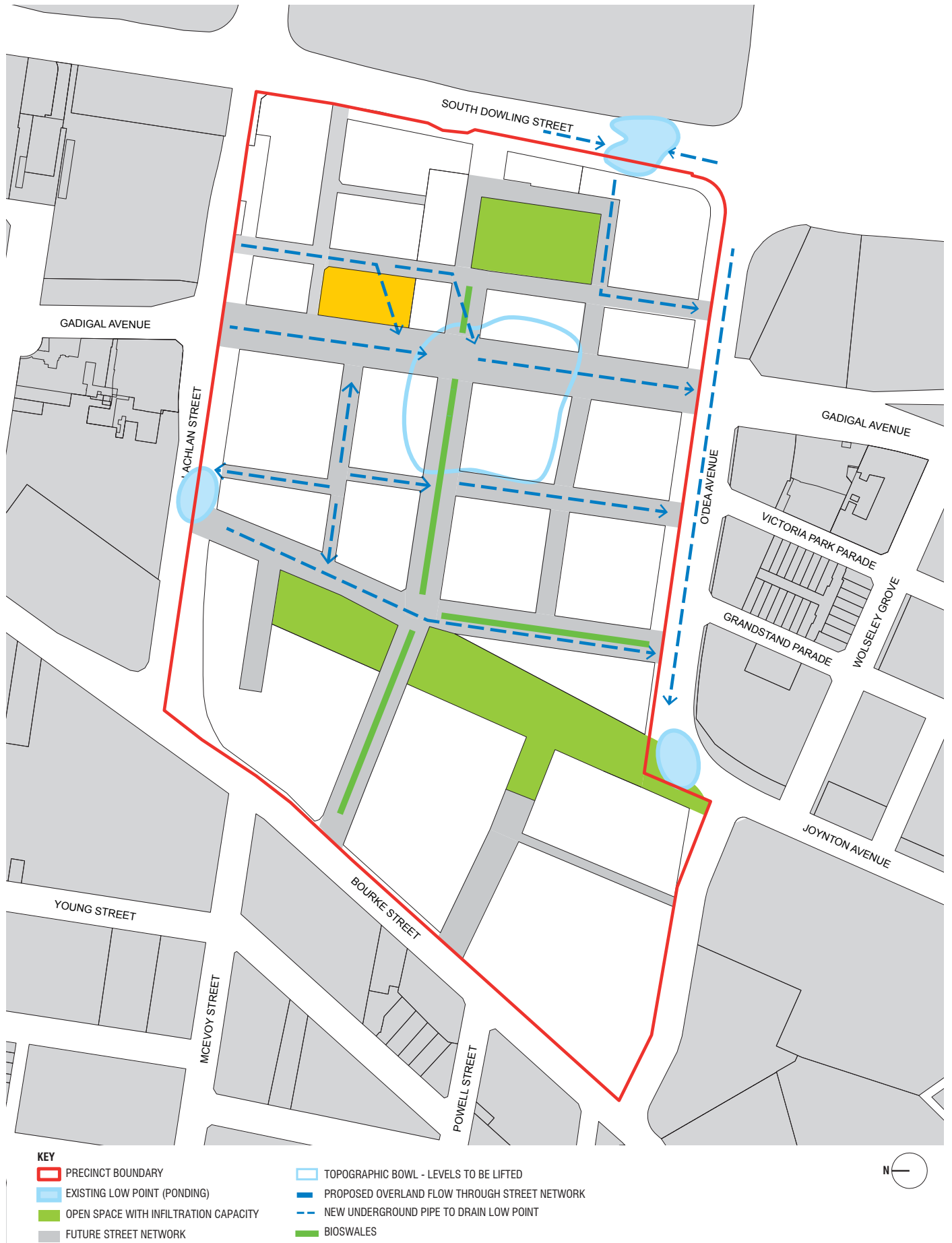
Figure 5.106 Lachlan Precinct Stormwater Management
