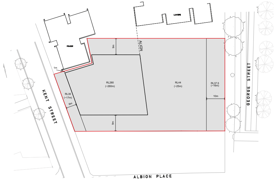
Figure 6.116 Minimum Building Heights & Setbacks for 505-523 George Street
